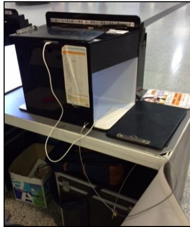
Lock wire set-up to ensure the box is attached with the table
